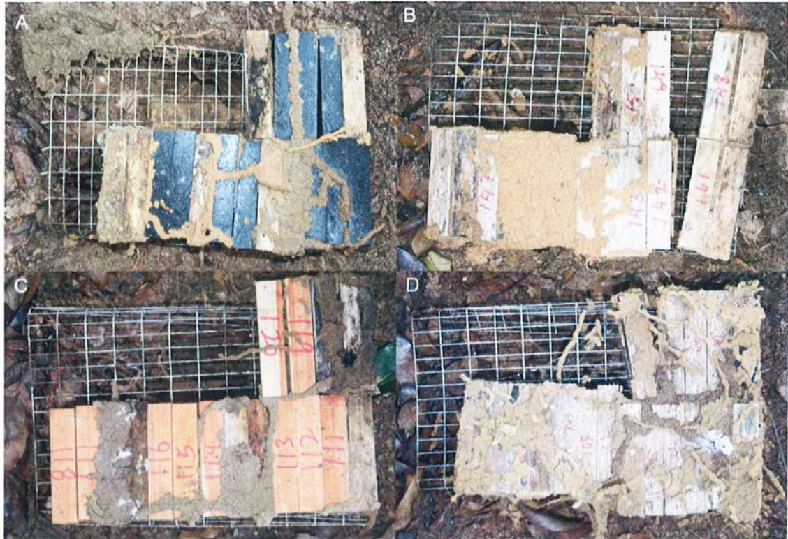
Figure 6.3 The four tested woods at the end of the 16 weeks of field test. (A) Maica's Compact Laminates. (B) Rubberwood. (C) Pinewood. (D) Particleboard.
