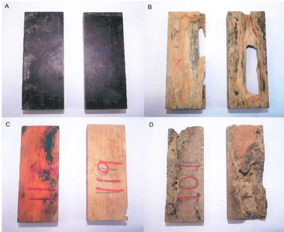
Figure 6.2 Test blocks after 16 weeks of field test. (A) Maica's Compact Laminates (Average visual rating=0). (B) Rubberwood (Average visual rating=2). (C) Pinewood (Average visual rating=0). (D) Particleboard (Average visual rating=2).
